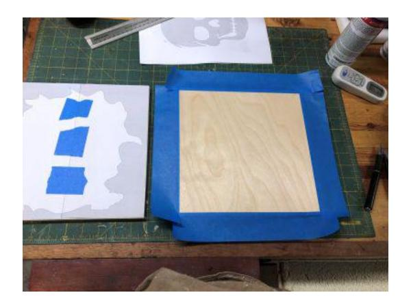
Tape the hole board pattern together for a full size pattern. Glue the pattern to the hole board.
