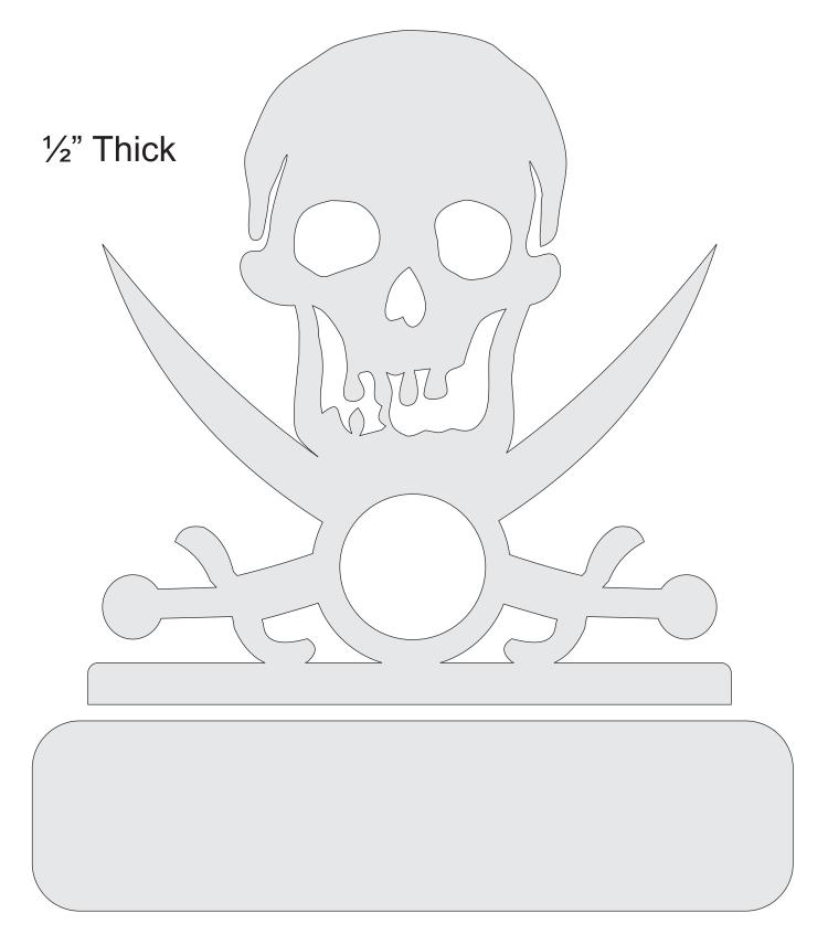
Requires a 1 7/16" Mini clock insert. Use a 1 3/8" Forstner bit for the clock hole.
