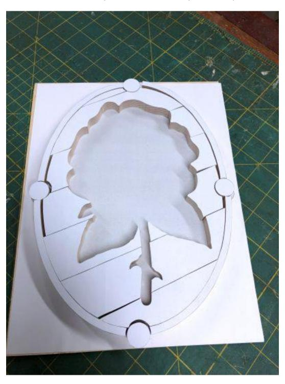
I used a #3 blade to keep the kerf as narrow as possible. This helps make the pieces fit well.
