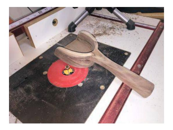
Use a 1/4" round over bit around the bottom of the scoop.
