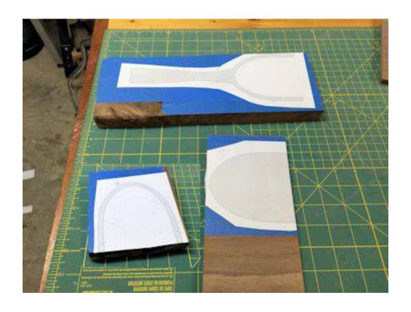
You will need 3/4" and 1/4" thick stock. Prepare the blanks with the patterns. Carefully cut all three parts.
