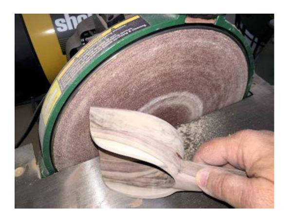
Sand a bevel on the bottom of the scoop to make it more efficient.
