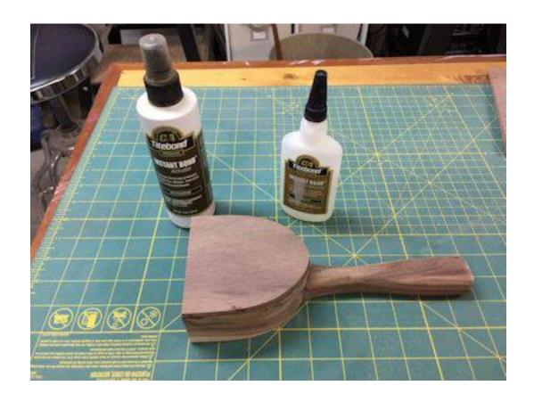
Glue the bottom to the scoop and sand it flush.
