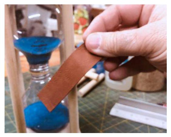
I used leather to cover the screws of the bulbs. You can use whatever you have. Just cut it to length and width and CA glue it around the screws.
