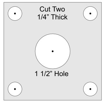
Center hole may need to be adjusted to fit the bulb you use. If the bulb sticks through to the other side the hole is too large.
