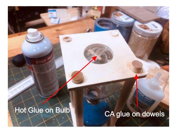
Insert the wooden dowels in the top and bottom holders. You can cut and sand them to the exact length after they are glued in place. At this point just make sure everything is straight.
