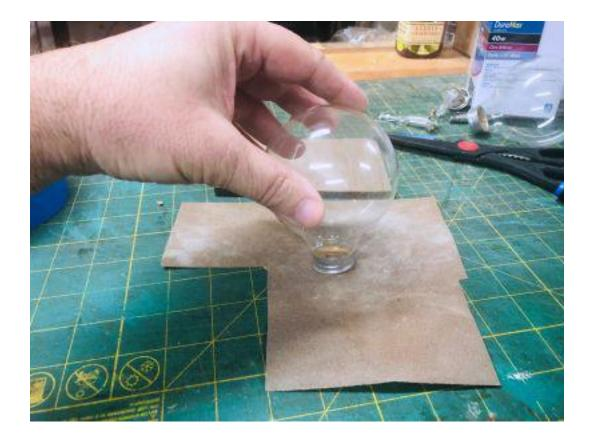
If the bulb does not sit flat the use sandpaper on a flat surface to make it flat and level.
