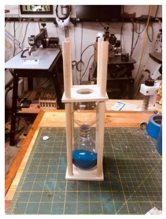
Capture the glass bulbs between the interior top and bottom.
