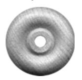
Wheel: 1-1/2" diameter 1/2" thick 1/4" hole 4 required
