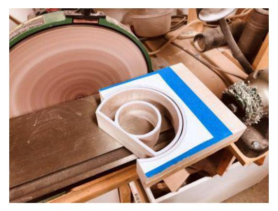
Cut the drawer away from the box walls then sand until the drawer rotates freely inside the box walls. Do this step before you cut out the walls.
