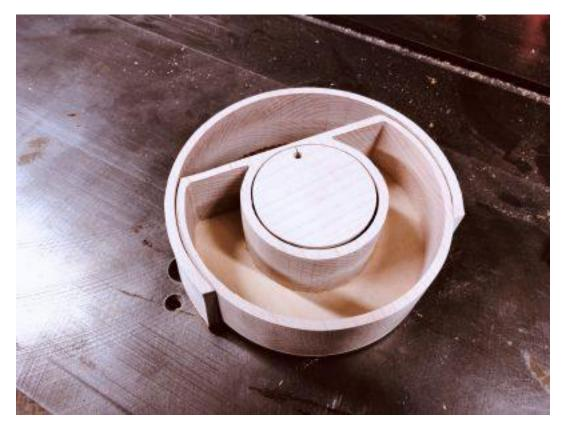
Glue in the center pivot while continuing to check that the drawer rotates freely. Sand as necessary.
