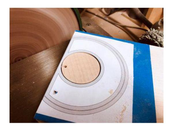
Sand the pivot until it rotates freely in the drawer.
