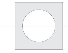
Drill 1/4" hole for dowel rod.
