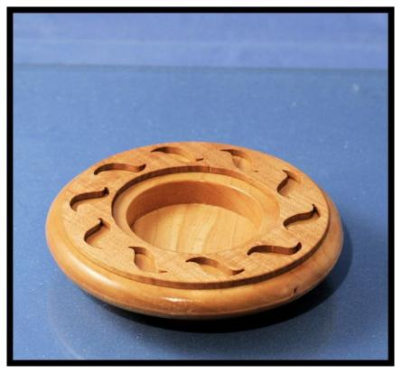
Roundover the top and bottom of the body with a router or by sanding.
