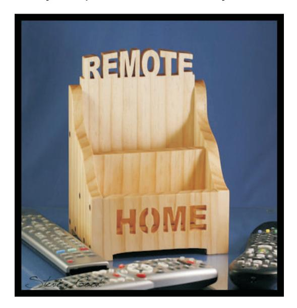
The dowels are mostly decorative and could be left out. I drilled the holes in the side walls before assembly. After glueing the project together I drilled the holes 1/4" deeper and inserted the dowels. They were sanded flush.
