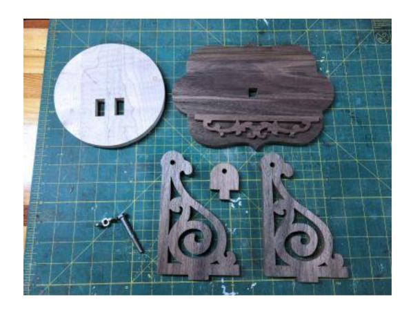
We will use a 2" bolt and wing nut for the adjustment shaft.
