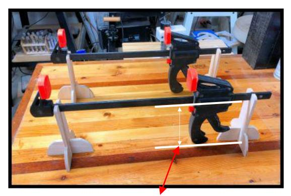
Measure the length from the bottom of the bar to the end of the handle. You need to choose the pattern that will allow the handle to not touch the table once installed in the stand.
