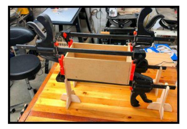
Once the project is elevated and clamped you can set the clamps in the stands. Now you have access to all four sides for extra clamps.
