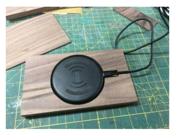
The charger is approximately 3/8" thick. I used 1/2" thick wood for the center body so I shimmed the charger to get it as close to the top as possible.
