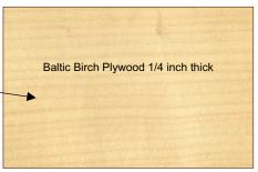
Use the spray adhesive to bond the jig saw template the 1/8 inch Baltic Birch Plywood.
