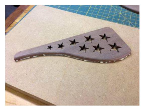
Carefully glue the segments back together. Only apply glue on the lower part of the piece.
