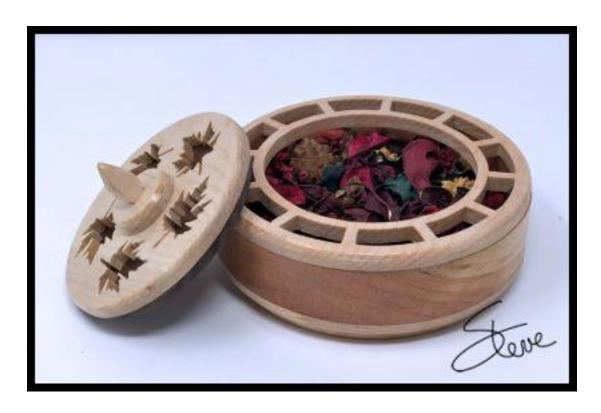
Notice that I rounded over all of the edges. I used a small round-over bit in my router table. You can also round over all the edges with sand paper.
