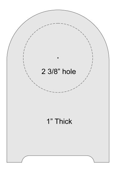
Insert hole is best cut with a 2 3/8 forstner bit. If you do not have one that size you can cut the hole with your scroll saw. Just cut slightly inside the line and sand to a snug fit. One advantage of the forstner bit is you do not have to cut the hole all the way through. This give the back a better apperance.
