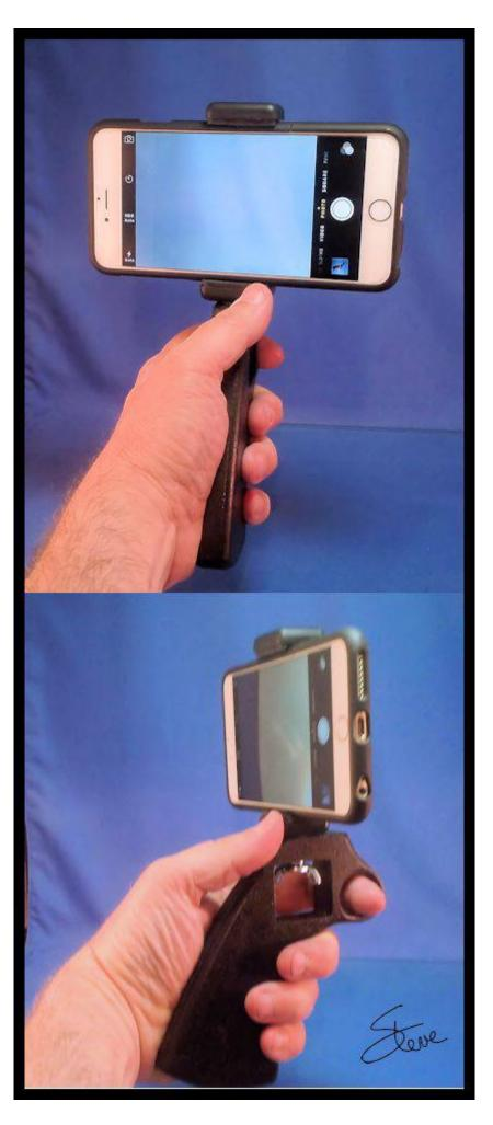
Required hardware: 1/4" 20 TPI 3/4" long wing screw. One 5/16" Neopreme washer.
