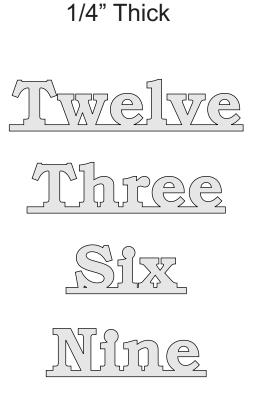
These are pretty small. I uses a #3 blade to cut the letters. I also used a micro drill bit to drill the entry holes. If you are very accurate you can drill the entry holes with a 1/16" drill bit.
