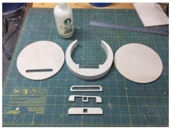
Cut the parts and prepare to sand and glue them together Glue the sound deflector over the cut out in the front. Clamp and let the glue dry.
