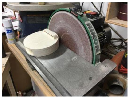
Carefully sand the bottom until you get ~ an 8 to 10 degree angle. If it's easier you can cut this on your table saw.
