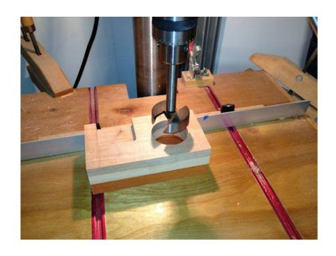
Drill the sound holeat the dimple mark. Drill to a depth just short of all the way through. Leave about a 1/4". If you do not have a large forstner bit you can use you scroll saw and cut the holes from each plate before the glueup.
