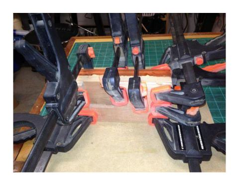
Clamp the glueup together and let it cure. After dry remove any glue squeeze out and sand all the sides flush.
