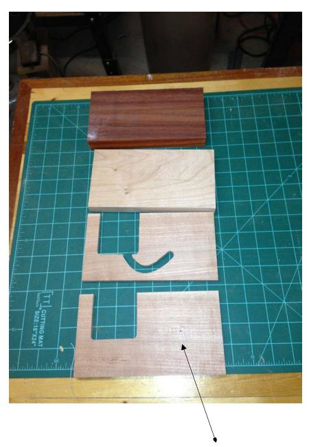
Cut out all the pieces. Notice the dimple showing the location to drill the hole in the front plate.
