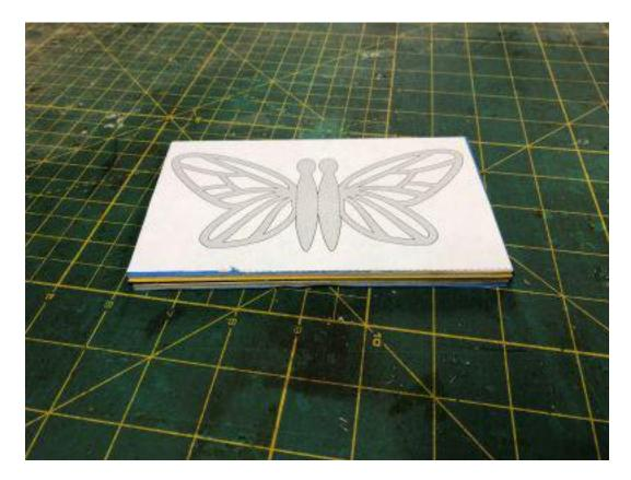
Wrap the stack of plywood and sheets of paper with blue painters tape to hold them together.
