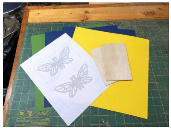
This technique is called sandwich cutting. We will stack all the sheets of paper between two pieces of 1/8" Baltic birch plywood.
