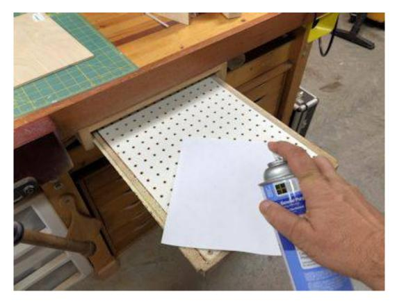
I normally use a pull out tray for applying spray adhesive. If you don't have one then the Spray Paddle is for you.
