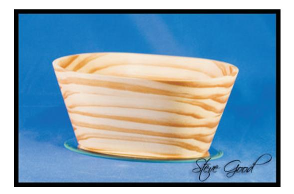
Drill the starter holes at 20 degrees. Set your scroll saw table at 20 degerrs. Start from the center ring and cut each oval. Stack and glue the concentric rings to make bowl.
