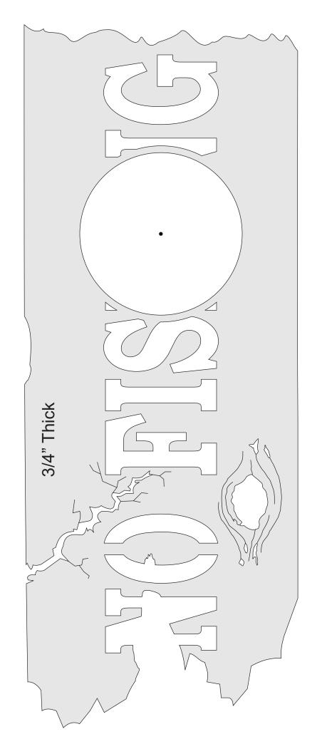
fit. It's better to make the hole too small than too large. do the other interior cuts. If you use your scroll saw cut just inside the line to make sure you get a good If you use a forstner bit, cut the hole before you
