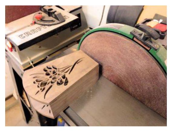
I'm using my disk sander to flatten the bottom. If you do not have a disk sander then glue a large sheet of sand paper to a flat surface. Move the vase back and forth on the sand paper until the bottom is flat. Ocasionally sit the vase on a known flat surfave to test for flatness. Finish sanding all the sides and glue on the base. Finish as desired.
