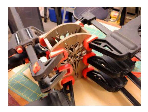
Glue and clamp the pieces. We will attache the base after the glue dries.
