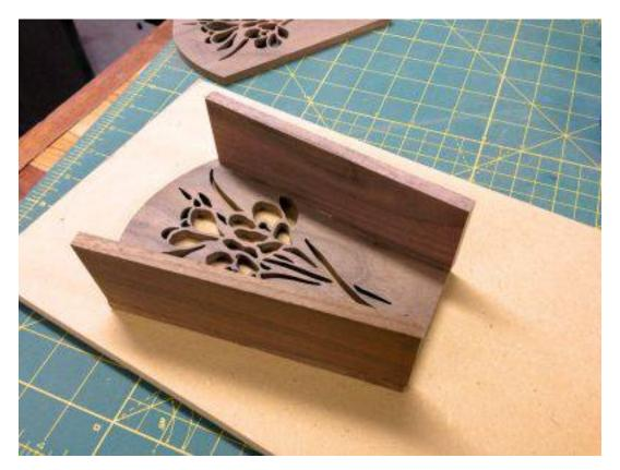
When you glue up the sides notice the angle on the bottom of the side piece. Let it over hang. We will flatten the bottom after the glue dries. This is easier than trying to cut the angle.
