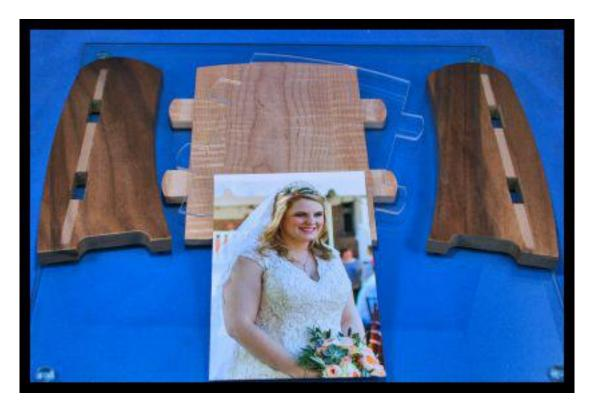
When you cut the slots for the tabs make sure you end up with a tight fit for the tabs and the acrylic sheet. The fit will hold the frame together. This way you can knock it down to remove the picture.
