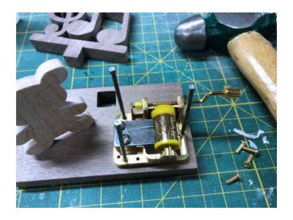
To mark the holes for drilling I used nails. The screws that come with the music movement are machine screws, not wood screws so you need to drill first.
