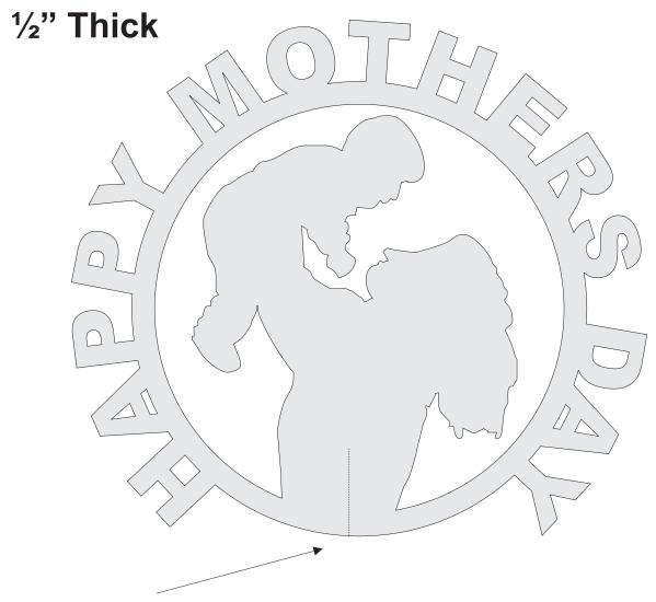
Drill 1/4" hole for dowel rod
