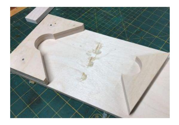
After the glue up dries you can remove the hot glue with a chisel or scraper.
