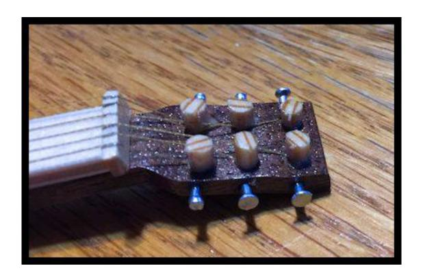
Cut some small nails to about 1/4" long. Drill six 1/16" diameter holes in the head stock. Super glue the nails in to the holes for tuners. Sand the dowels until the are about 1/16" long.
