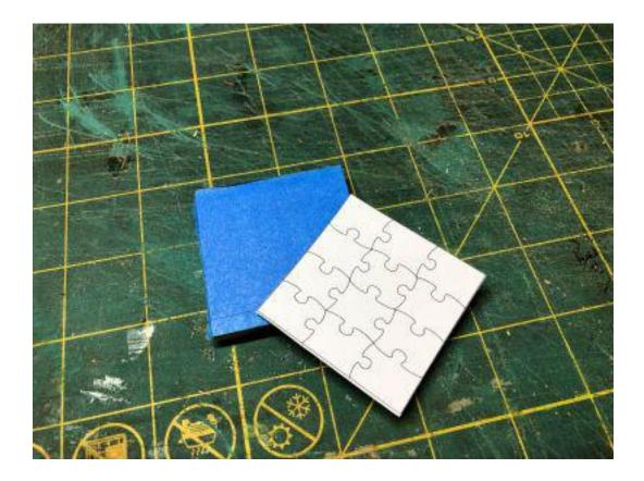
Wrap the stack in blue painters tape. Glue the puzzle template to the top of the stack.
