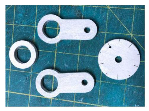
Since all the parts are 1/4" thick you may need to slightly sand the roller thinner so it rotates easily.
