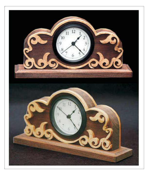
The main body of the clock is 1 inch thick. Use a 3 1/4 inch hole saw to cut the clock insert hole first. Then you can use a 1/4 inch contrasting wood glued to the bach of the clock. This should be the same as the wood used for the front scrolled decoration. This gives the clock visual balance. After the piece dries apply the pattern making sure the pattern is aligned with the clock insert hole. The crown is optional. Simply cut it away if you don't like it.
