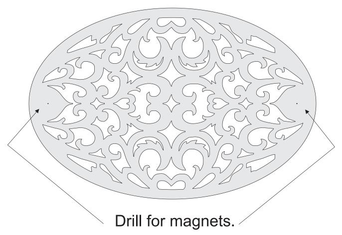
Adjust the thickness of the wood to your magnets. Also adjust the holes for the magnets.
