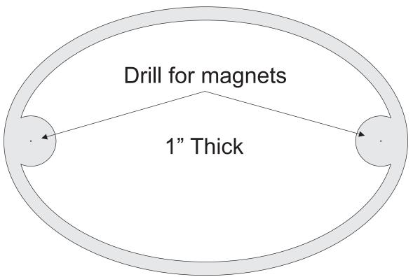
Make sure to epoxy the magnets in place with the correct polarity so the lid is attracted to the bottom.
