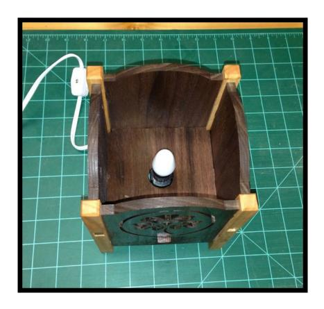
The light kit installs in the 1 inch hole. The socket is spring loaded and just snaps in.
