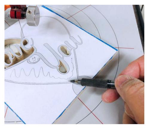
We talked about the fragile parts in interior cut 7 and 8. To prevent breaking while you make the remainder of the do not remove the waste after you cut 7 and 8. Just move the blade to the next cut and let the waste help hold the piece together.
