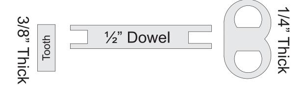
After glue in the tooth drill a 17/64" hole in the end of the key.
