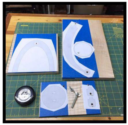
Lay out all the parts on the wood blanks. Drill the 1/4" holes in the neck and the shade brackets.
