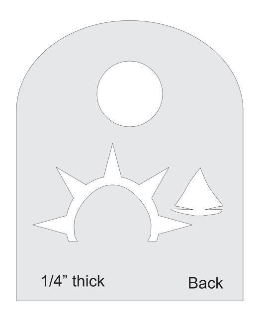
Use a 1 3/8" forstner bit to cut the hole for a 1 7/16" mini clock insert.
