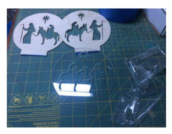
Make sure you remove the protective cover from both sides. You can lightly sand the edges with 220 grit sand paper if they are a little tough.
