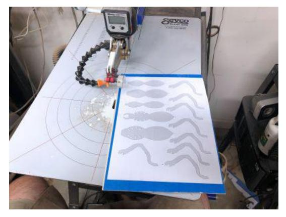
The small version of the pattern uses 1/8" thick Baltic birch plywood. This wood can be difficult to cut. It is easier to stack cut two or more.
