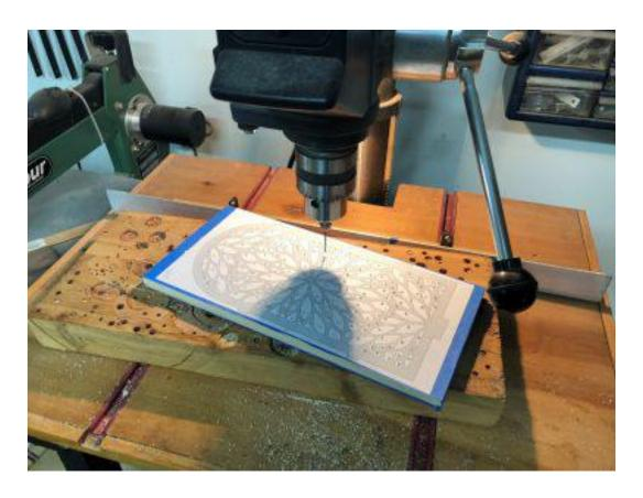
Here are all four sheets of the 1/8" Baltic birch plywood stacked together and bound with blue painters tape.
