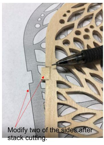
Stack cut all four sides with the pattern with the tabs. We will mark and cut the tabs off of two of the sides after we complete the stack cutting.
