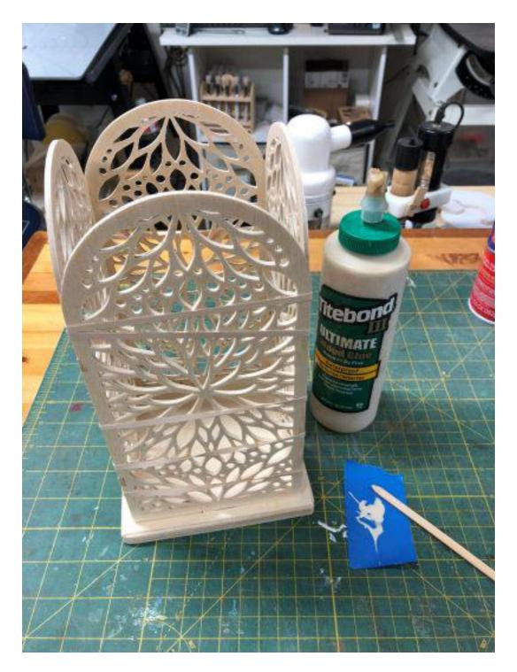
Glue all the slots into the tabs and secure with rubber bands until the glue dries.
