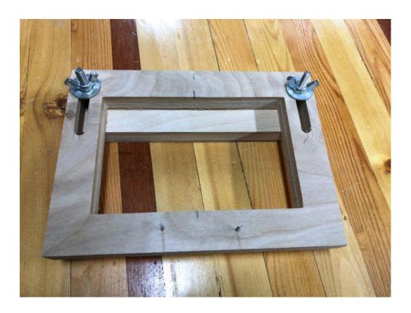
Small nails are driven just slightly through the jig to hold the project in place while the keyhole slot is cut. These nails can be driven in different locations depending on the shape of the project.
