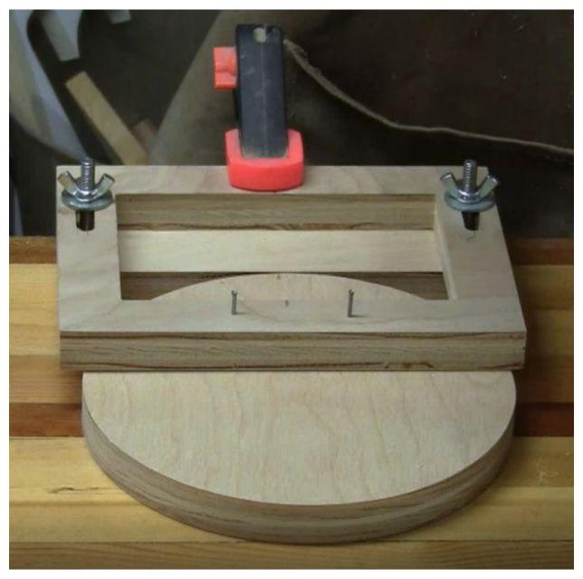
The jig is clamped to the workbench. The project is slid under the body of the jig and against the fence. The small nails lock the project in place to the slot can be routed.
