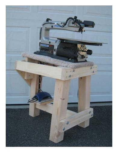
The rear leg is angled back 5 degrees. The front legs are angled 5 degrees to each side, but aren't angled forward in order to keep the design simpler, and to not interfere with the operator's ability to sit/stand closer to the saw.
