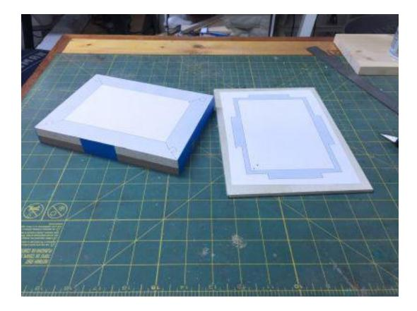
Use blue painters tape to stack the two 1/2" thick boards together. We will stack cut the frame.
