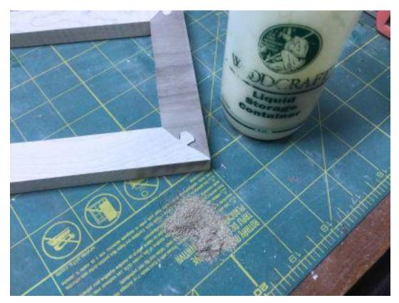
I'm going to use the saw dust from the cut to make wood filler.
