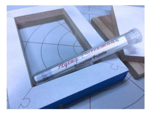
For the miters we need to use a very thin blade. I am using the Flying Dutchman Superior Puzzle blade. You could substitute that blade for a #2/0 blade.
