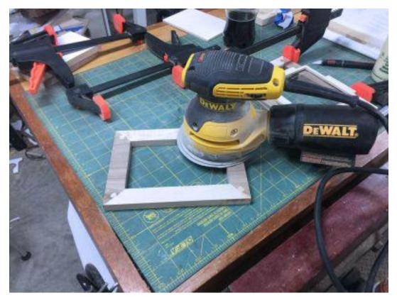
After the wood filler dries you need to sand it flush. Give the whole frame a good sanding. Ease over the edges and prepare for finish.
