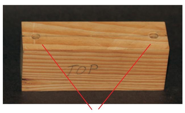
Drill holes on a center line. Drill Block A 1/4 inch. Drill Block B slightly larger for play
