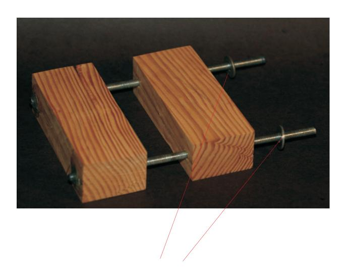
Install a washer on each rod
