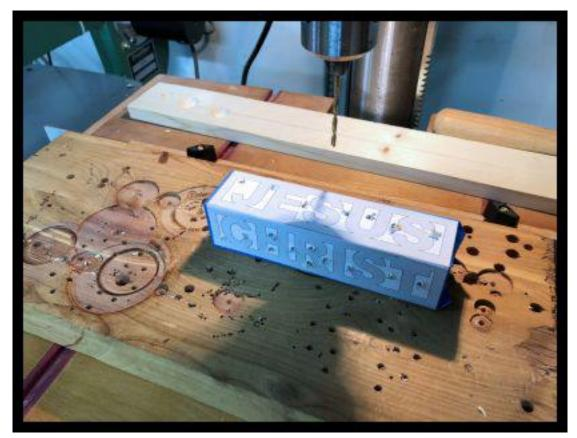
Drill the entry holes on both sides of the pattern. It's best to try to keep the entry holes centered.
