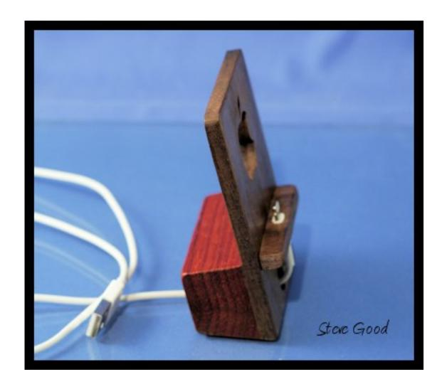
The bottom was sanded to a 15 degree angle after it was glued up. I used a disk sander with the table set to 15 degrees to do this.
