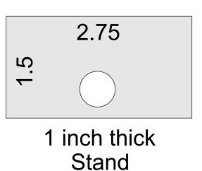
Cut the connector hole then use a small file to file to a snug fit.
