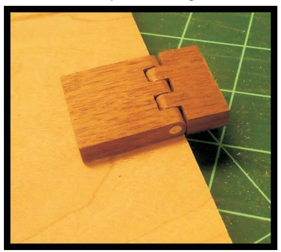
Notice I sanded the dowel flush with each side of the hinge.
